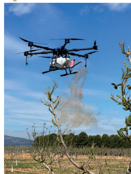
Drone applying pistachio pollen on the crop. Photo: Quino Cayuela.
